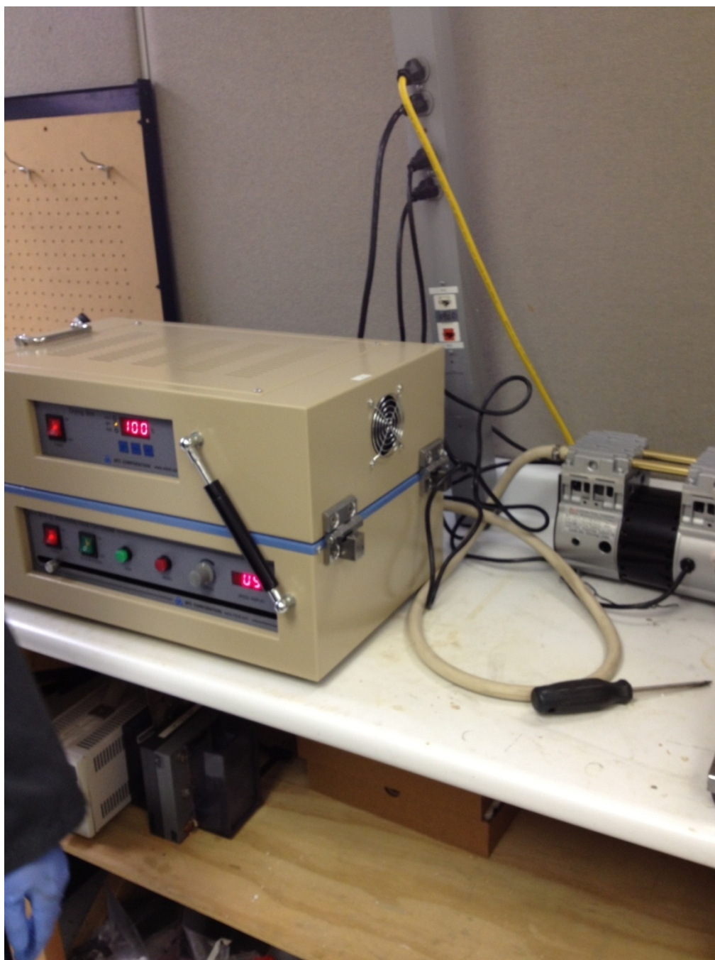
Figure 8. Baking Cathode Material
