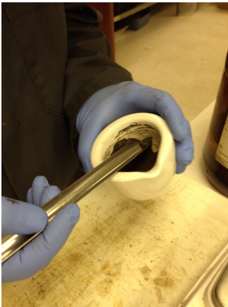
Figure 1. Lithium Manganese Dioxide Produced by Double Controlled Heat Treatment of Chemical Manganese Dioxide From American Manganese Artillery Peak Material mixed with Lithium Carbonate
