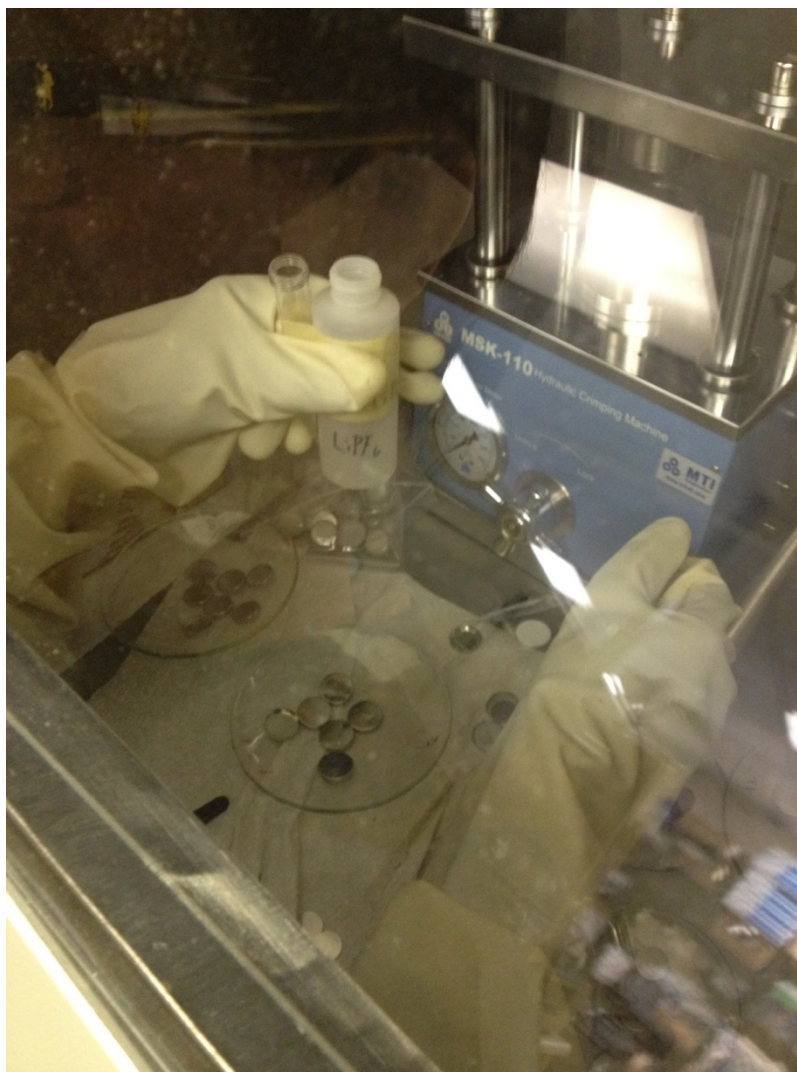
Figure 10. Assembling Button Cell in Controlled Humidity Chamber
