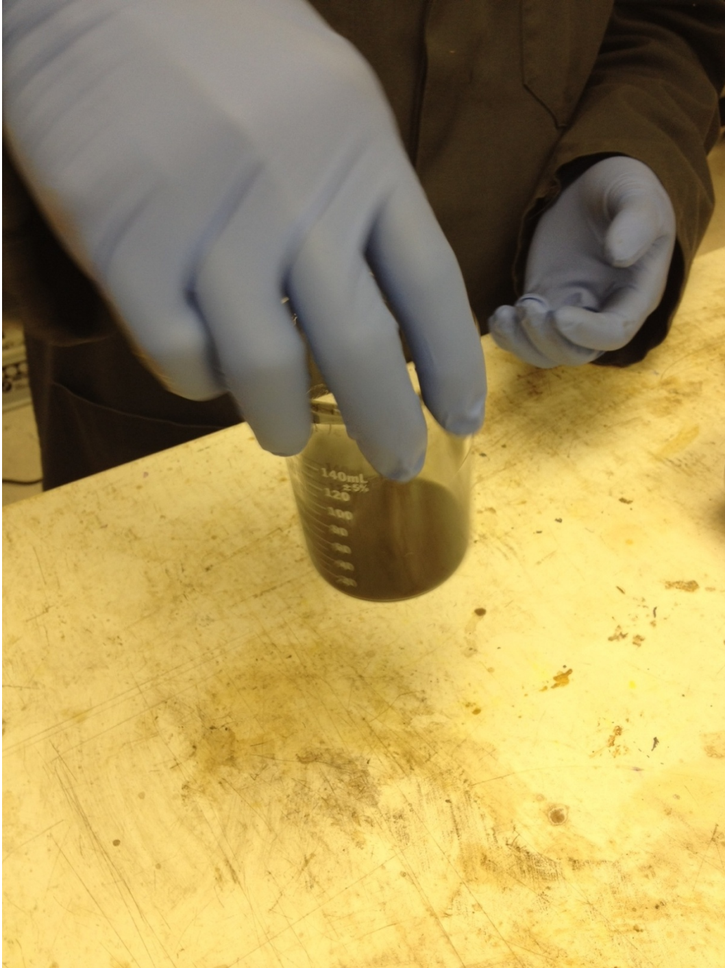
Figure 4. Mixing Cathode “ink”
