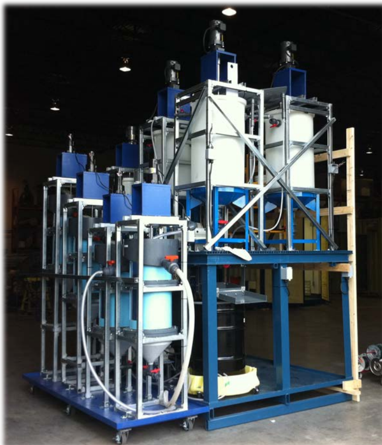
Figure 1 - Electrolytic Manganese Dioxide Recovery Process for Low Grade Manganese Ores
